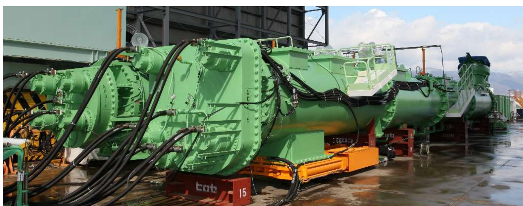
Φ1.5 m screw conveyor (No.2 and No.3)
