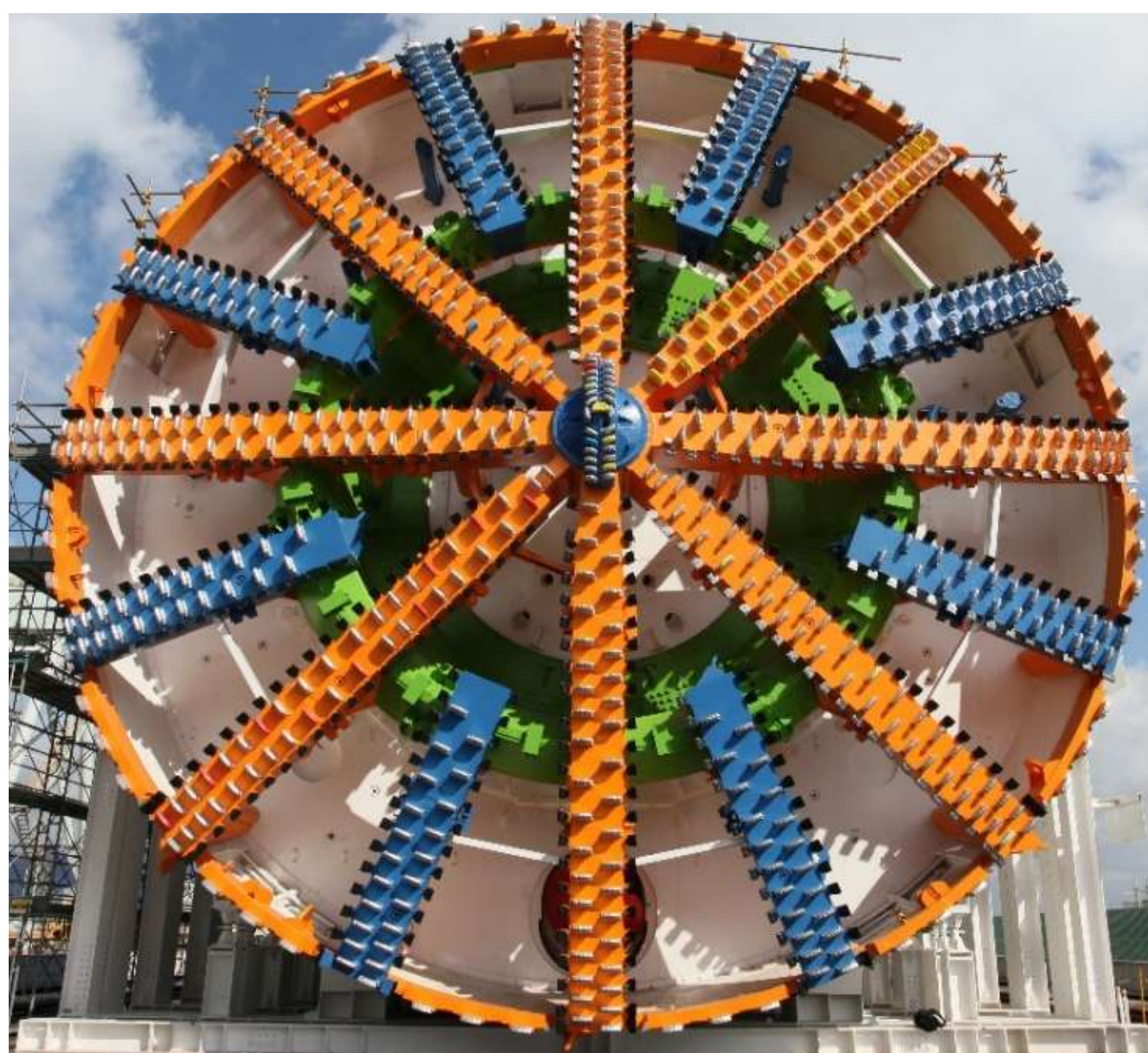
Cutter head front view (66.4% opening)
