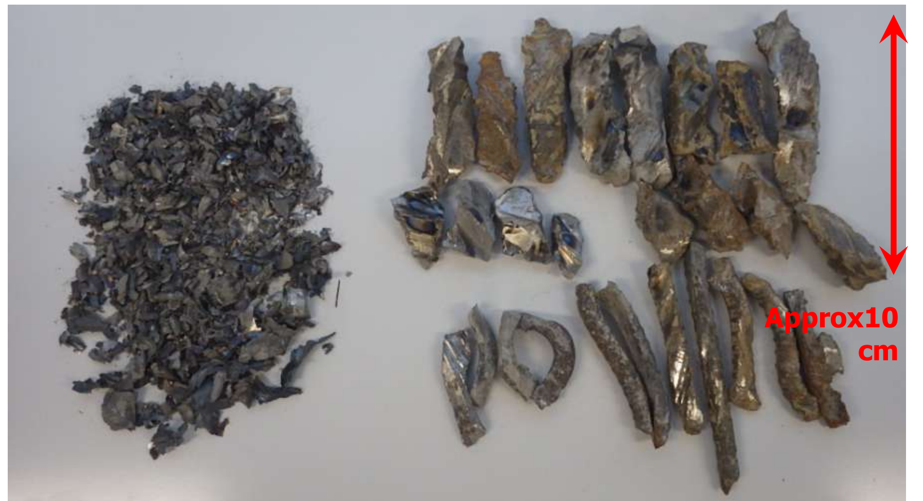
Steel reinforcement debris after pile cutting
