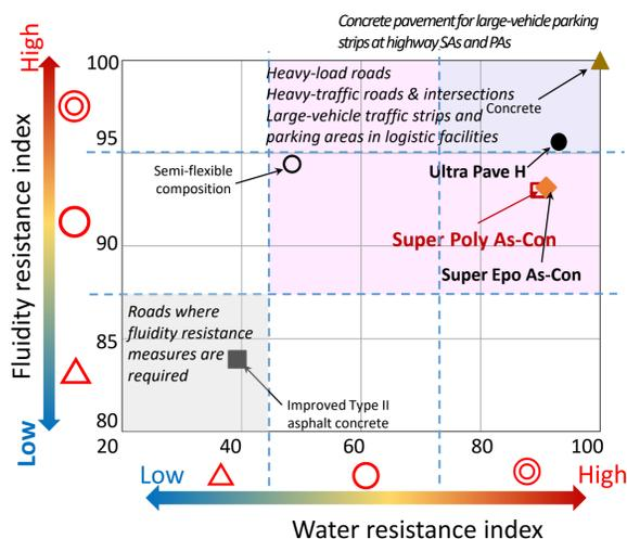
Fluidity resistance and water resistance indices based on HWT test results with the base of concrete pavement as 100
