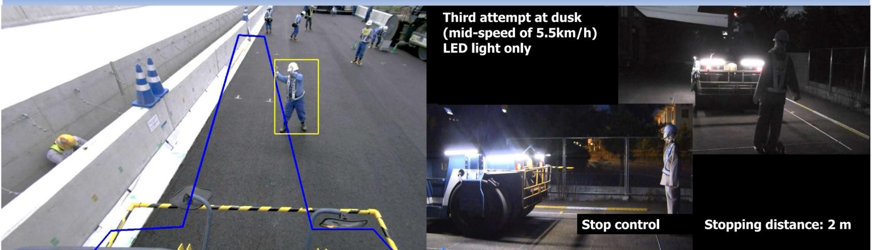
The advanced image analysis system will detect human presence even when only a person's foot gets inside the defined detection area. The yellow frame shown above indicates that the system has recognized human presence in the control distance range so that the vehicle will be automatically slowed down by the control unit.
