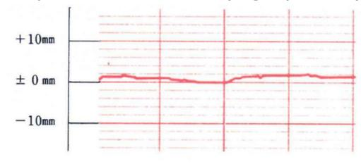
Example of flatness measurement result (using 3 m profile meter)
