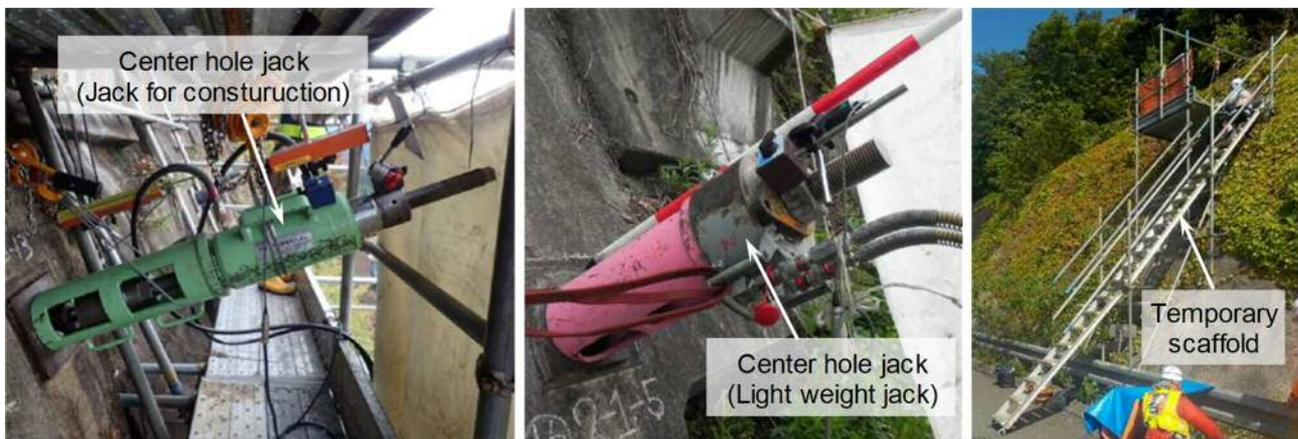
Photograph 1 Center hole jack and scaffold used for lift-off test
