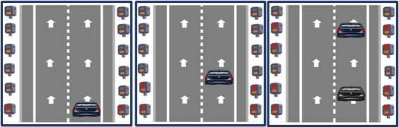
Figure 10 - Diagram of the operation of detector beacons in low visibility conditions. A-8 Motorway. Alto del Fiuoco (Lugo). Spain
