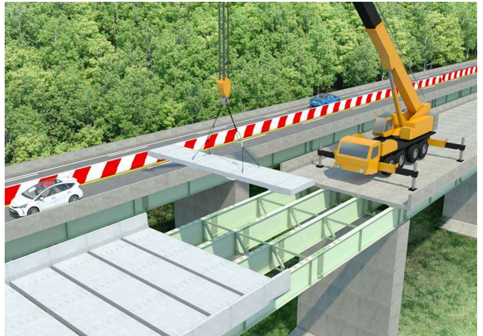
Precast deck slab jointing
