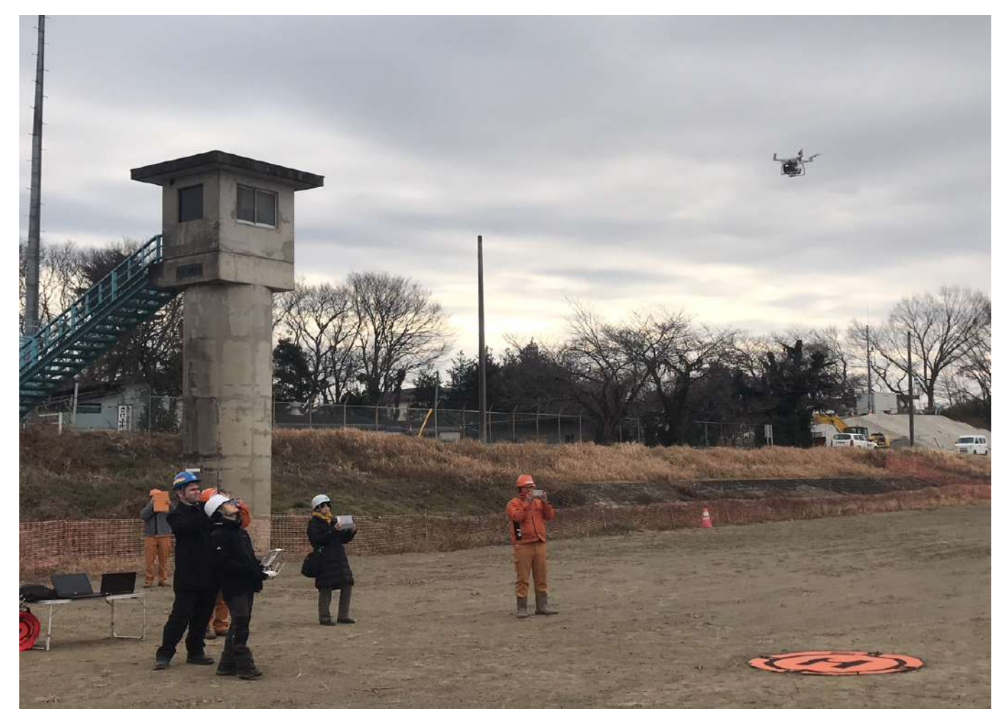
Measurement operation using the GCP-less UAV system
