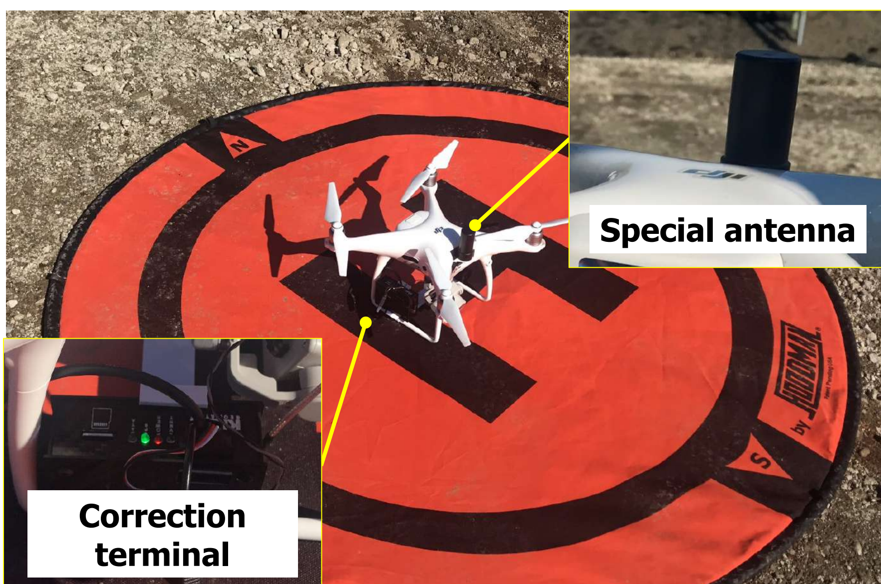
Aircraft for GCP-less UAV
