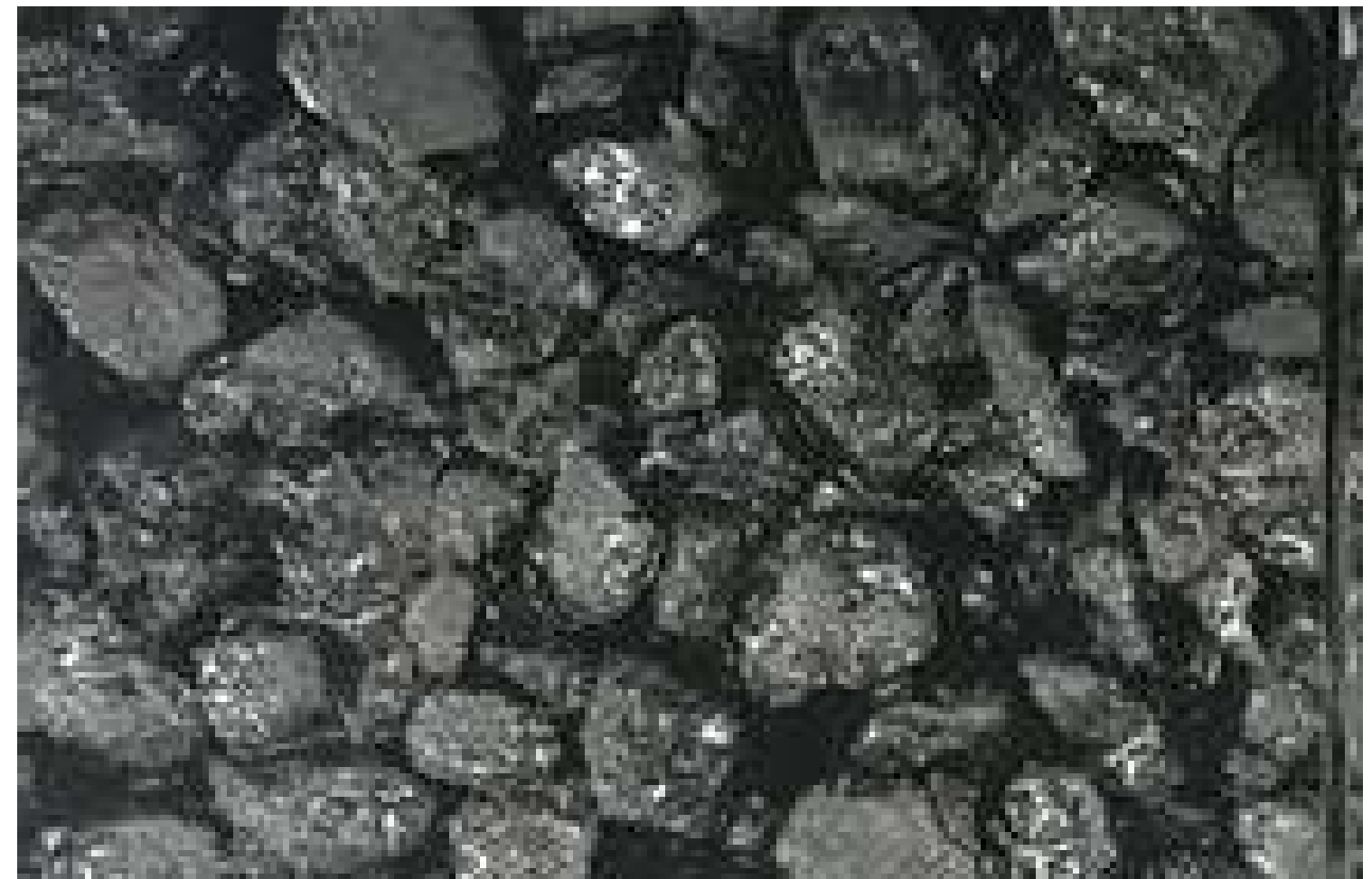
Conventional porous asphalt with conventional binder
