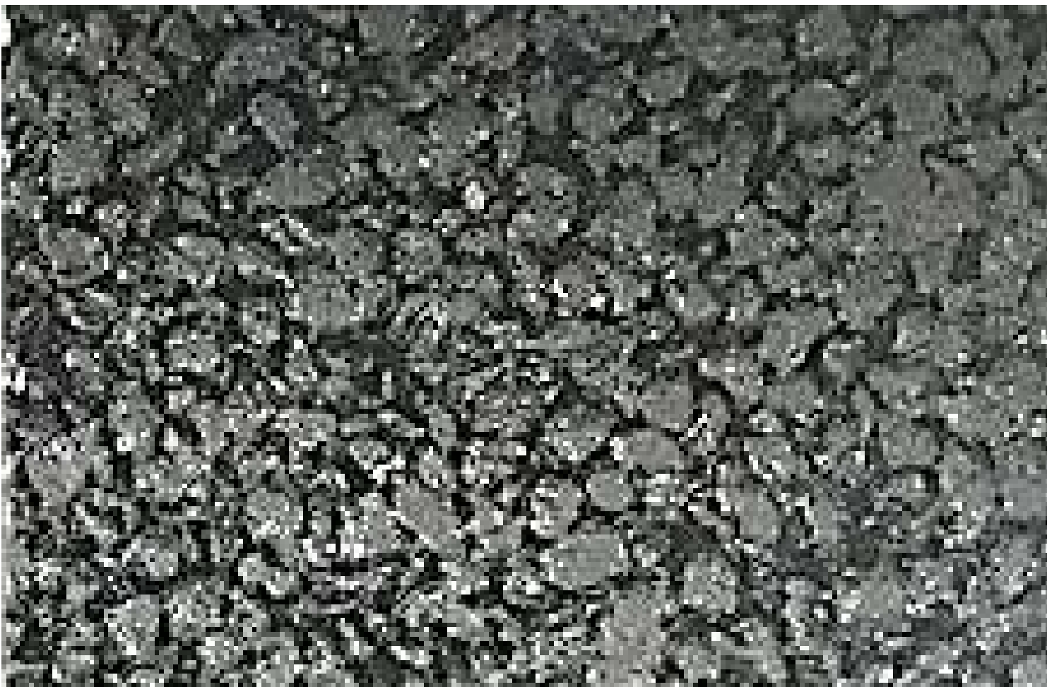
Smaller aggregates porous asphalt with TOUGHPHALT SUPER MX
