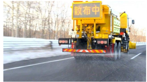
Improving the efficiency and performance of snow and ice operations by optimizing the amount of salt spraying
