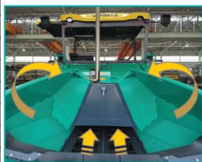
Hopper and feeder
