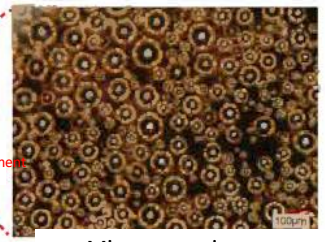
Microscope image (spherical shapes indicate air bubbles)
