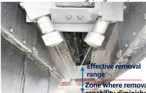
Collision nozzle jetting
