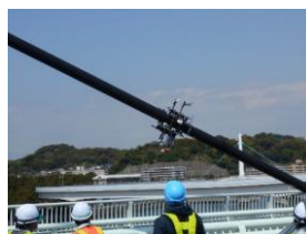
Imaging using a cable robot
