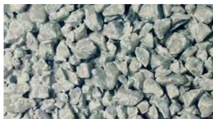
L-size (Aggregate grain diameter: 5 - 13 mm)
