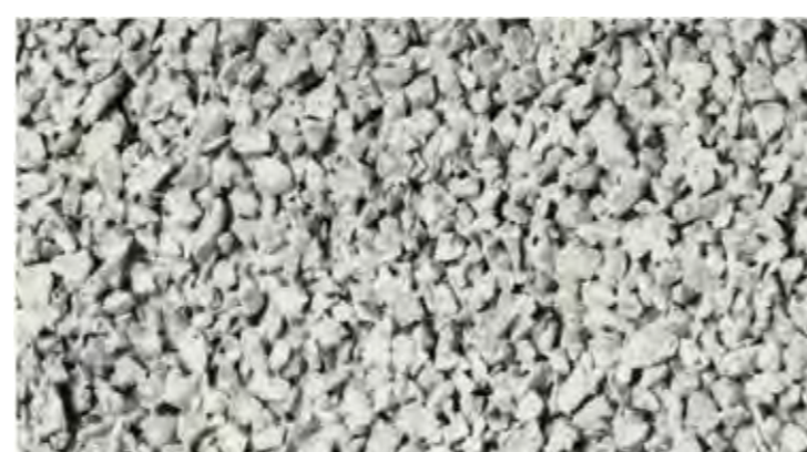
M-size (Aggregate grain diameter: 2.5 - 5 mm)
