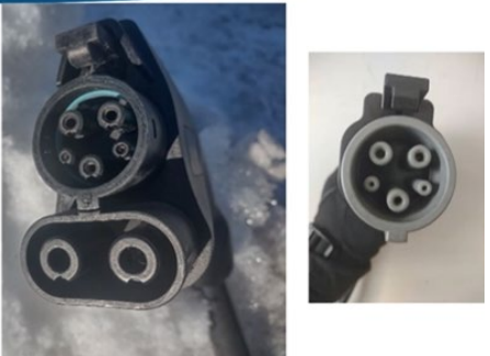
Left: CCS Type 1 Connector, Right: J1772 Connector Photo Credits: FHWA
