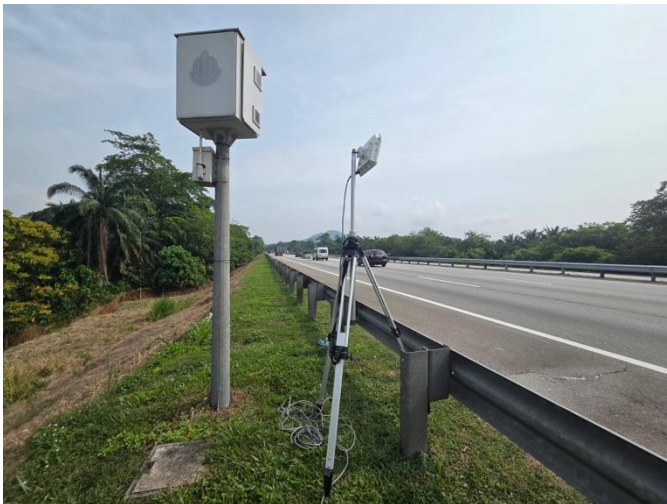
Figure 1: Smart Sensor microwave-based traffic detector set-up at a fixed speed-camera measurement location.
